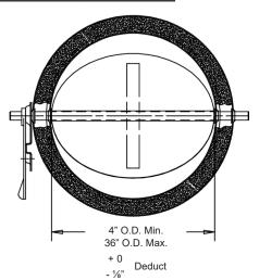
Damper fits inside both skins of dual wall spiral duct. Note that O.D. and I.D. are 1/6" undersized.
